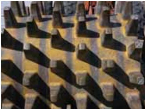
Figure 5.3: Sheepsfoot rollers compact soil.
